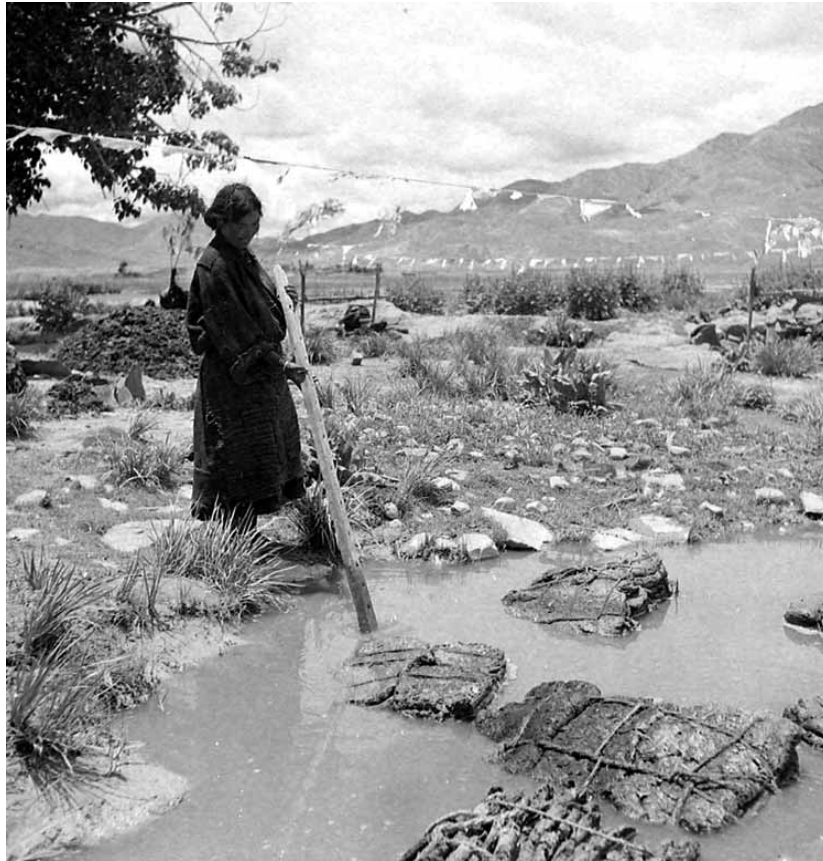
Figure 22: Soaking the Mulberry bark for paper making.
